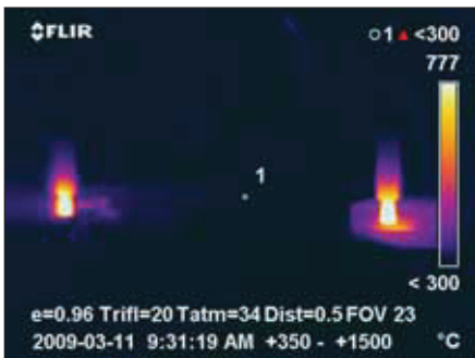
Figure 3: Thermal image of optimised funnel forming
