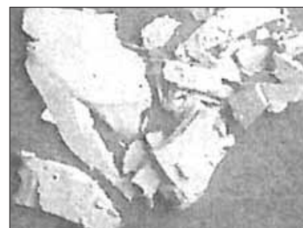
Figure 5: SEM image of flakes formed by delamination
