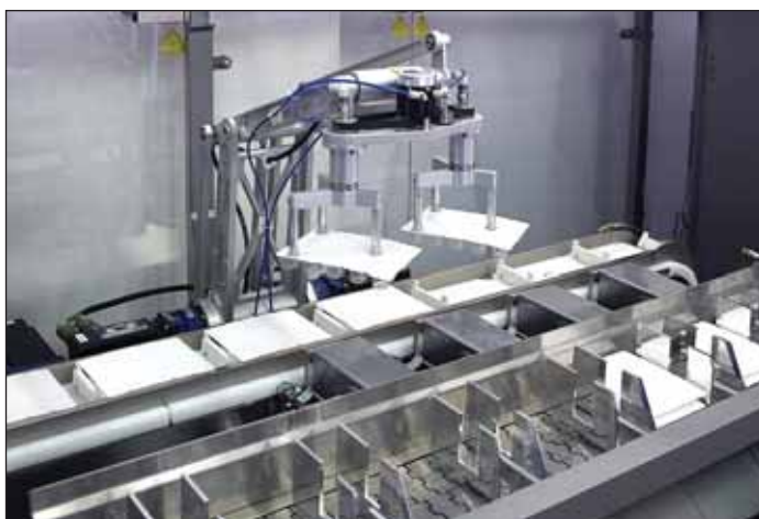
Figure 3: The Robocombi robotic feeder places syringe trays in the cartoning machine
