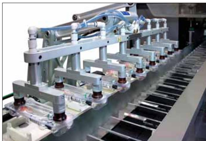
Figure 3: The Robocombi robotic feeder places syringe trays in the cartoning machine
