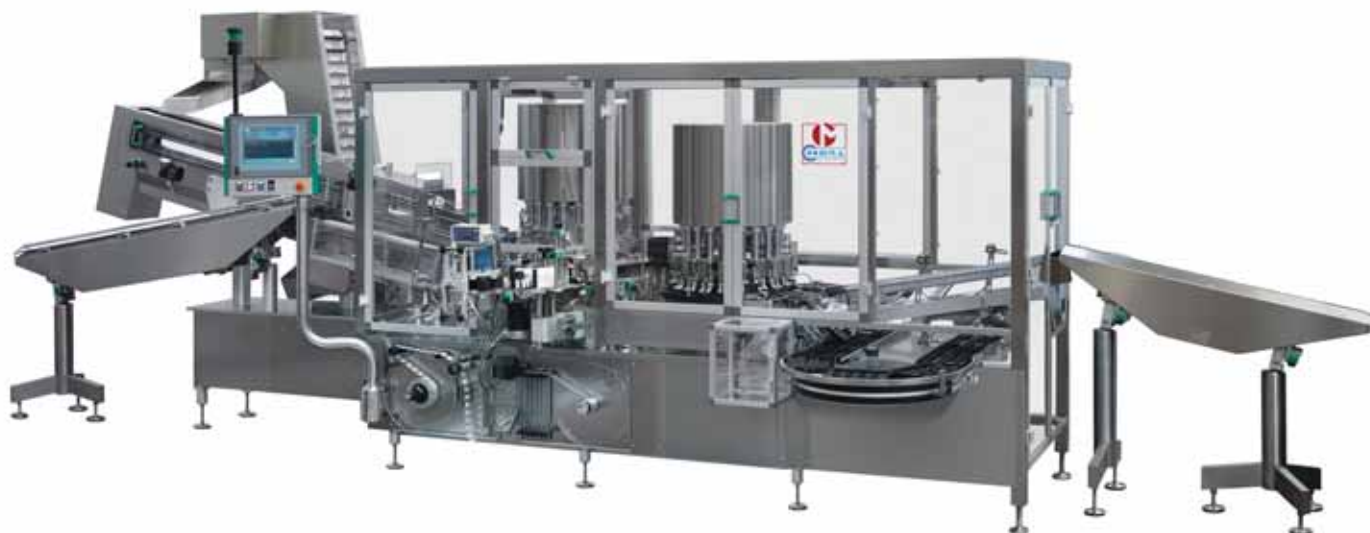
Figure 1: The Corima APS Combi syringe assembly machine
