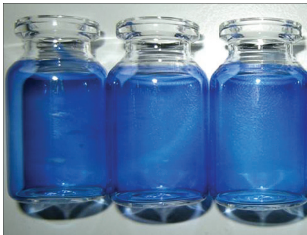
Figure 2: Result of Colouring Agent Test Showing Strong Colouration of Altered Glass Surface After Accelerated Ageing Test Using 0.9% KCl as Extraction Solution.
