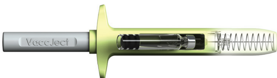
Figure 1: As the cartridge is inserted into the VaccJect device, the enclosed double-ended needle penetrates the cartridge septum, opening the fluid path for drug delivery.
