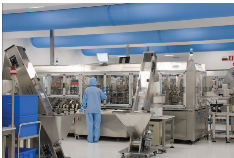
Figure 2: The cleanroom for MDI valves and nasal saline actuators is classified as ISO 7 ‘at rest’.
