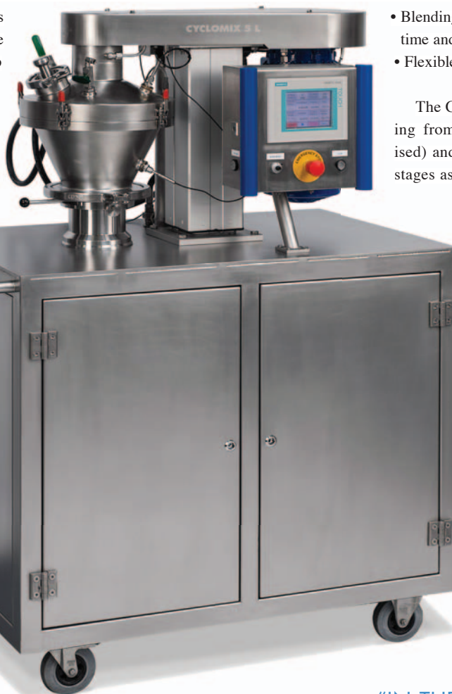
Figure 1: Possible configuration of a 5 L Cyclomix machine.
