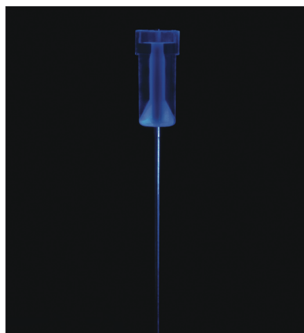
Figure 3: UV-fluorescent glue enhanced visual inspection process.
