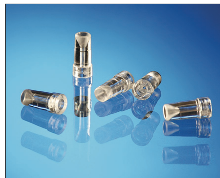
Figure 4: High precise injection moulding parts from the polymer material polycarbonate, produced from a 64-cavity tool with hot runner system.
