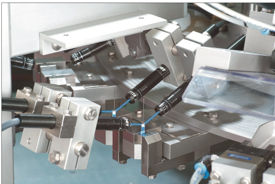
Figure 1: Fully automatic needle gluing, using UV LED lamps for the curing process
