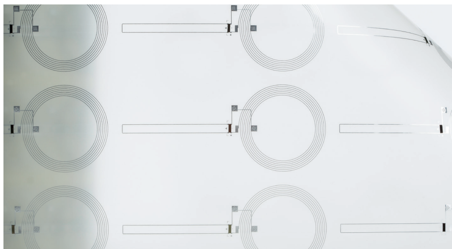
Figure 4: Thinfilm's sensor technology used in combination with YpsoMate Smart. The sensor is a printed integrated circuit for use in electronic read-only transponders (passive sensor). The tag transmits data (128 bits) at a frequency of 13.56MHz used by HF RFID and NFC (operating in a Tag-Talks-First manner). The code of the NFC signal changes as the linker of its antenna is physically disrupted. As such, the change in the NFC signal corresponds to the actual use status of YpsoMate Smart.
