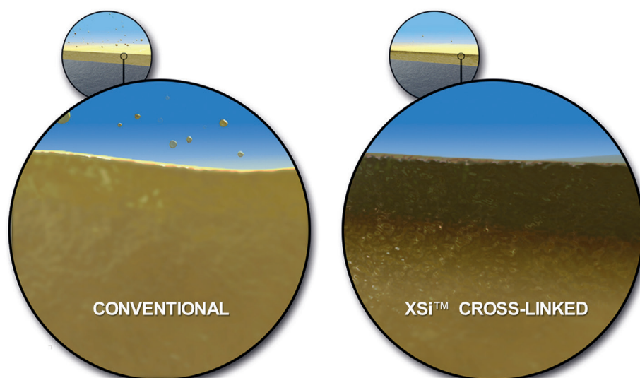
Figure 1: Conventional versus BD XSi™ cross-linked silicone chain networking. The modified lubricant layer acts as a barrier to silicone emulsification, reducing the migration of silicone oil from the barrel and maintaining the lubricity required for the syringe to perform as intended.
