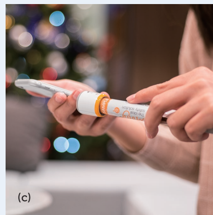
Figure 4: The connected, disposable Molly® C auto injector (a) with re-usable data recording and transmission device (b) which enables transmission to a smartphone via Bluetooth (c).
