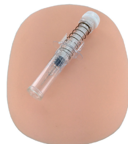
Figure 2: In the study, each user performed six injections on a silicone pad. (Safe'n'Sound® device shown here post-injection, i.e. in the safety-activated state).
