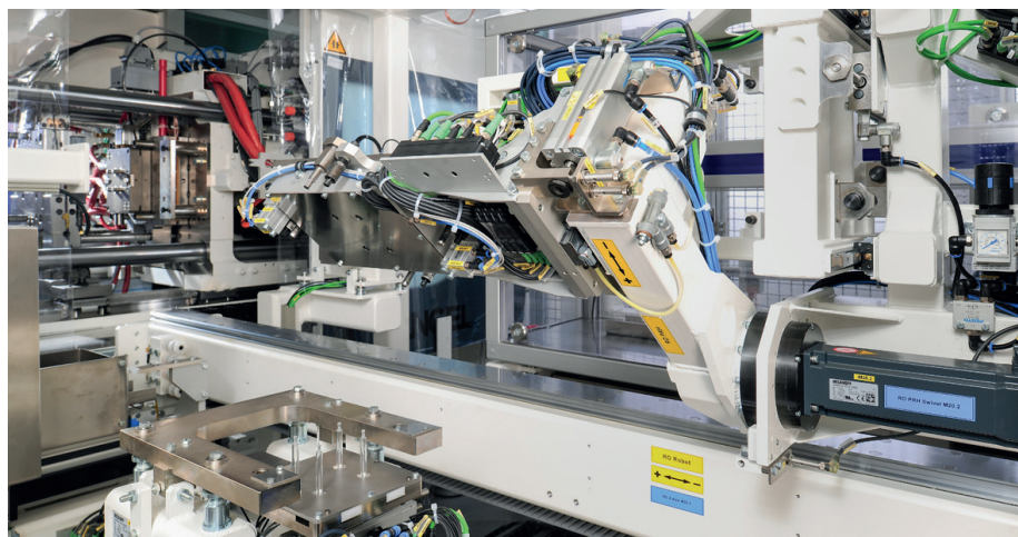
Figure 2: The take-out module includes a 4+4 insert, a take-out robot, and a shuttle system.
