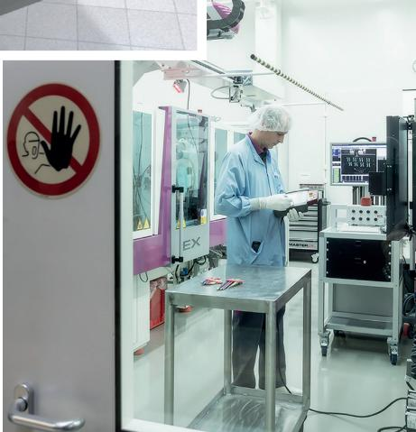
Figure 2: One of Trelleborg's Class 8 cleanrooms where safety-critical medical LSR components are produced fully automatically to a zero-defect policy.
