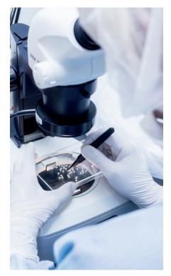
Figure 4: AQL inspection of micro parts in a Class 7 cleanroom environment.
