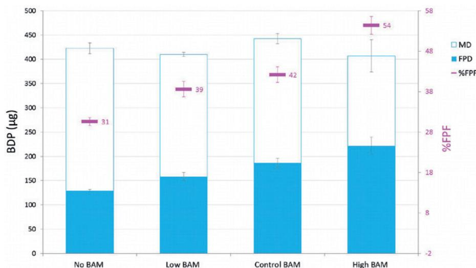
Figure 1: Impaction data shows that dose dispersion performance improves with increasing BAM set pressure; mean values (n=3); error bars ±SD.
