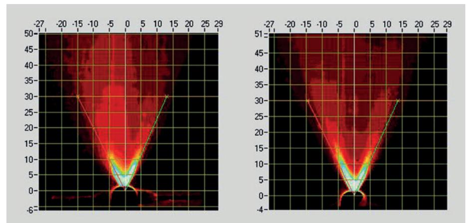
Figure 4: Example data from Plume Geometry (comparison of angle and shape of plume).
