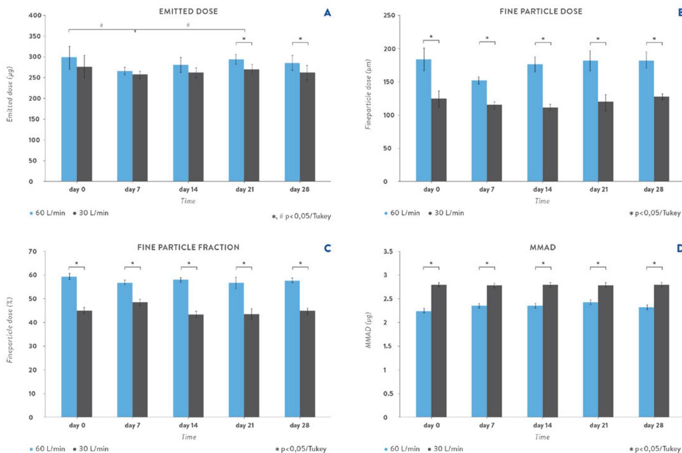
Figure 4: (A) Emitted dose ( $\mu\text{g}$ ), (B) Fine particle dose ( $\mu\text{g}$ ), (C) Fine particle fraction (%), (D) MMAD ( $\mu\text{m}$ ) of salbutamol sulphate at 30 and 60 L/min from a 2-pin standard inhaler (Mean  $\pm$  SD,  $n=6$ ). \* indicates significance between 30 and 60 L/min. # indicates significance between different time points at 60 L/min.
