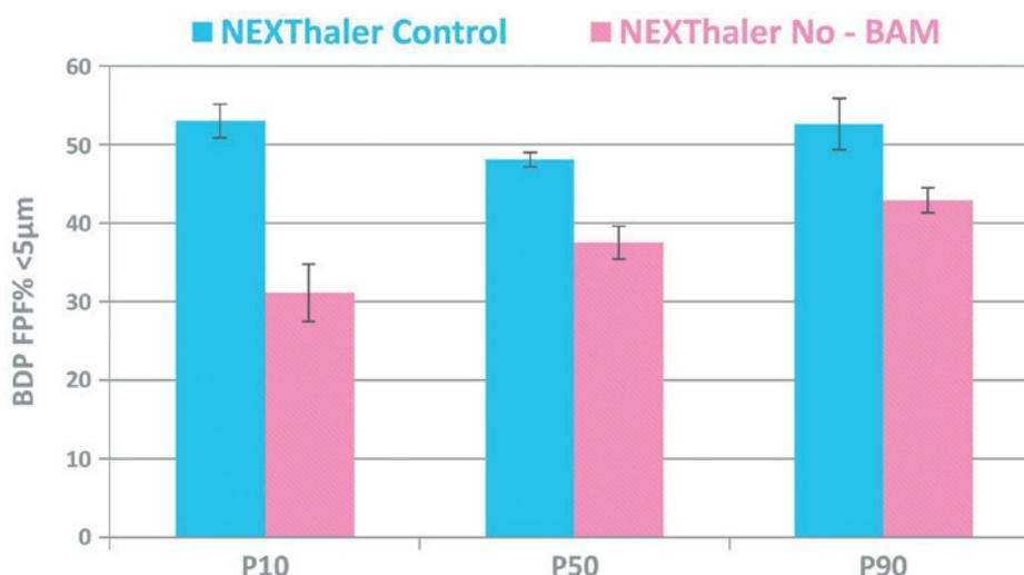
Figure 3: Incorporating a BAM in the DPI device improves the magnitude and consistency of the FPF% across a range of flow rates (n=3).
