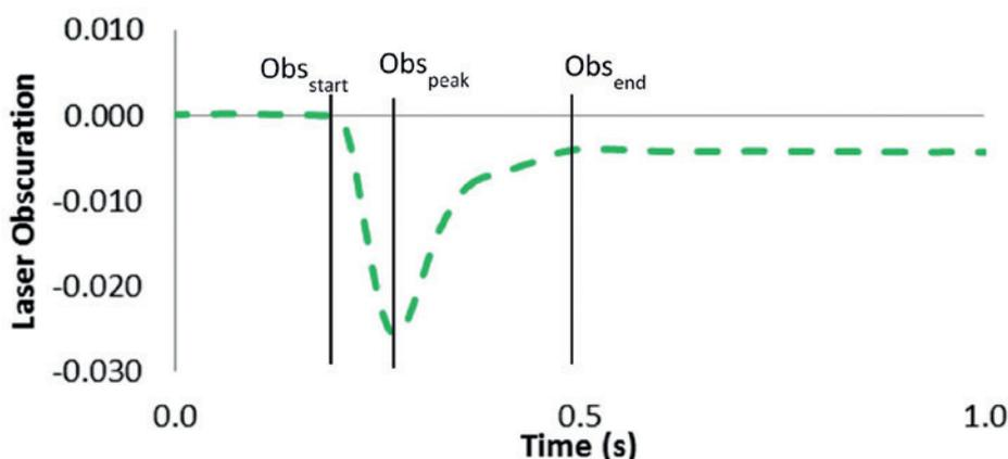
Figure 5: Dose evacuation data using the No-BAM device with the P50 inhalation profile demonstrating the start (Obs<sub>start</sub>), peak (Obs<sub>peak</sub>) and end (Obs<sub>end</sub>) of the laser obscuration, which characterise the dose dispersion event.
