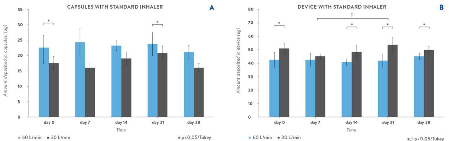
Figure 3: Deposition of salbutamol sulphate remaining in (A) capsules and (B) device, following aerosolisation at 60 L/min and 30 L/min from a 2-pin standard inhaler (Mean  $\pm$  SD, n=6). \* indicates significance between 30 and 60 L/min. # - indicates significance between different time points at 60 L/min. † indicates significance between different time points at 30 L/min.
