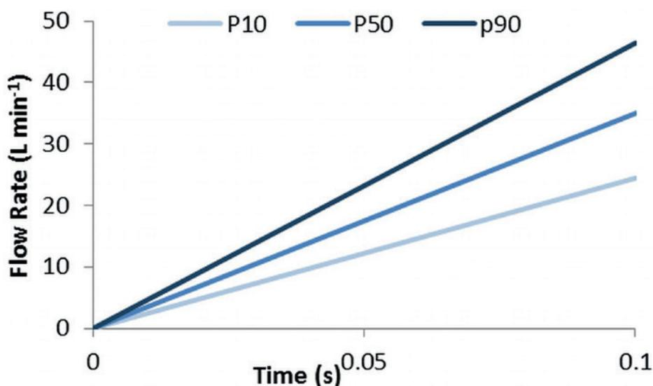
Figure 4: Increase in flow rate between 0 and 0.1 secs for the P10, P50 and P90 inhalation profiles; P90 is associated with the fastest acceleration rate.
