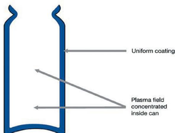
Figure 2: a) Traditional plasma processing does not ensure a uniform coating to internal wall of the canister whereas b) the new plasma process gives a uniform coating to canisters.
