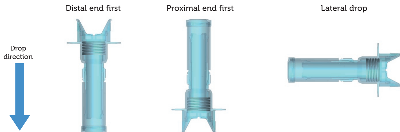
Figure 2: Safe'n'Sound® before syringe assembly, drop test without syringe.
