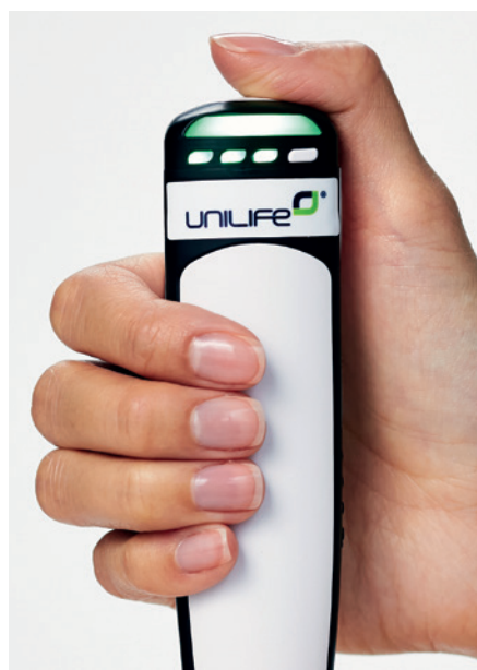
Figure 4: Unilife’s LISA™ platform of smart disposable auto injectors allows pairing of the device with Bluetooth LE connectivity as well as a related app.
