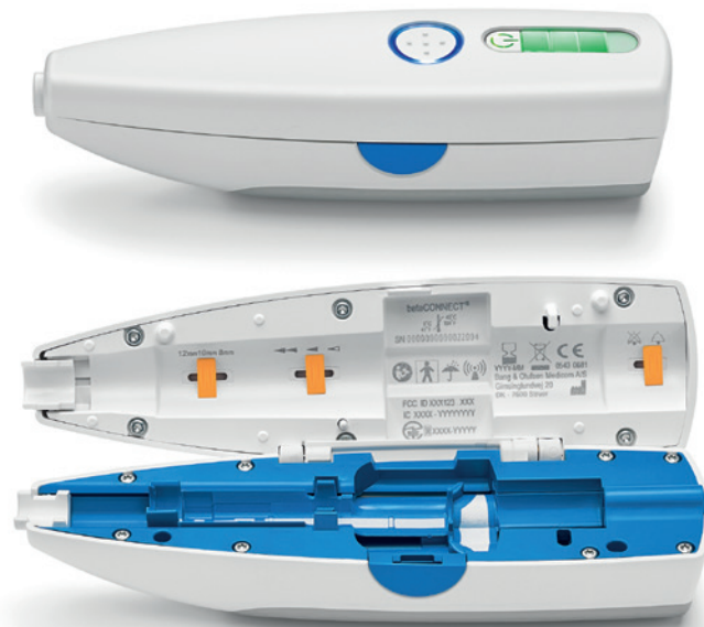
Figure 3: The BETACONNECT re-usable, fully electronic auto-injector can be used as part of a complete software-based system designed to track injection history and share important treatment information with healthcare providers. (Image courtesy of Bayer.)
