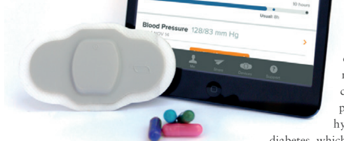
Figure 6: The Proteus platform comprises four elements: sensor-enabled pills, containing an ingestion sensor; body-worn patch (pictured) which receives a signal from the pill; the Discover App (pictured); and the Discover portal, for physicians. (Image courtesy Proteus Digital Health.)
