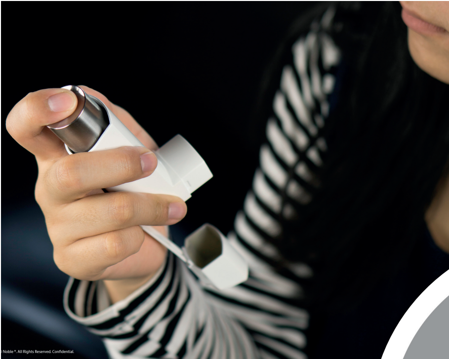
Figure 3: MDI training device designed to be true to form and function of an actual MDI.
