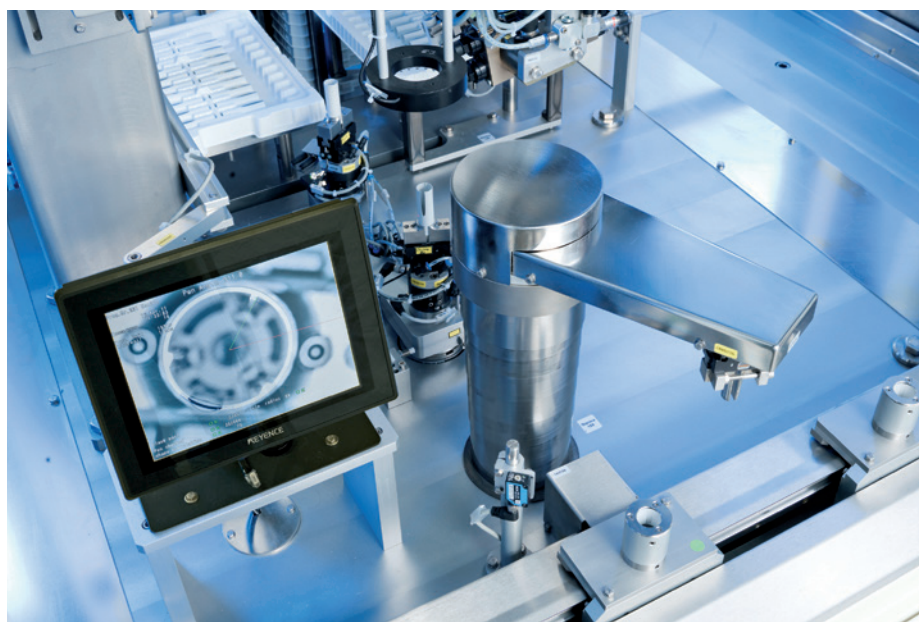
Figure 3: Testing and positioning the shell of an injector device.
