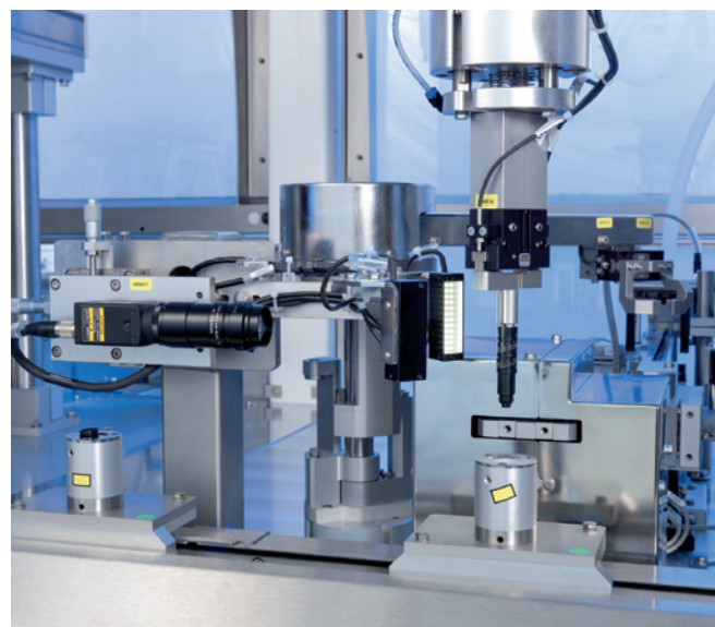
Figure 5: Testing and inserting the injector's dial.
