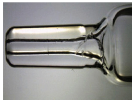
Figure 6: Spiral cracks with low fatigue strength called cone cracks can be found on the area where the cone meets the shoulder.
