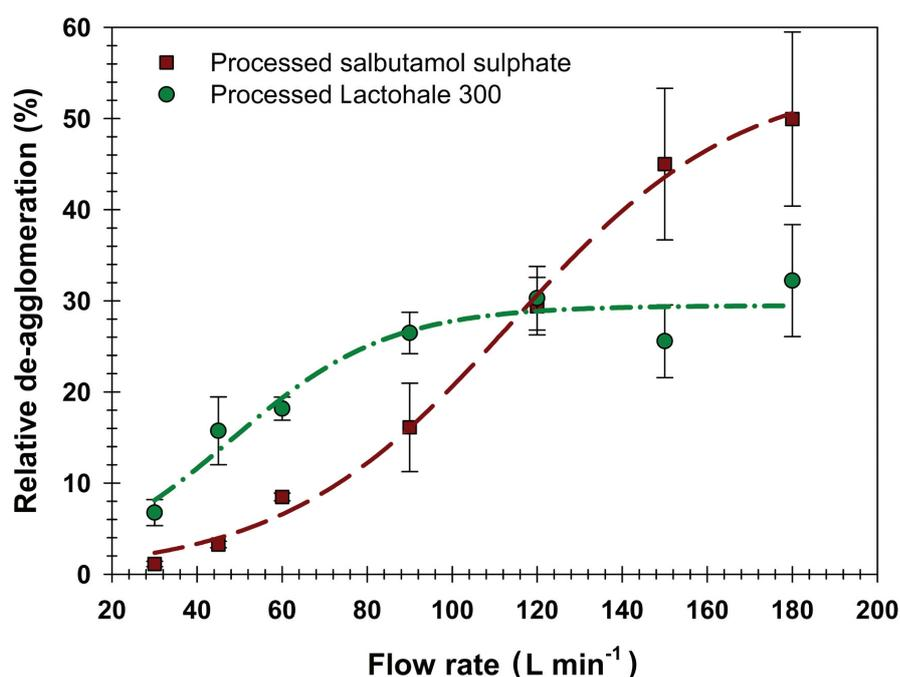
Figure 5: Relative de-agglomeration versus flow rate profiles for salbutamol sulphate and Lactohale 300, including empirical model curves.
