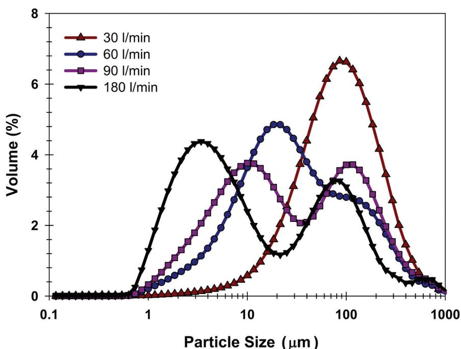
Figure 2: Particle size distributions for salbutamol sulphate measured at flow rates in the range 30-180 L/min.
