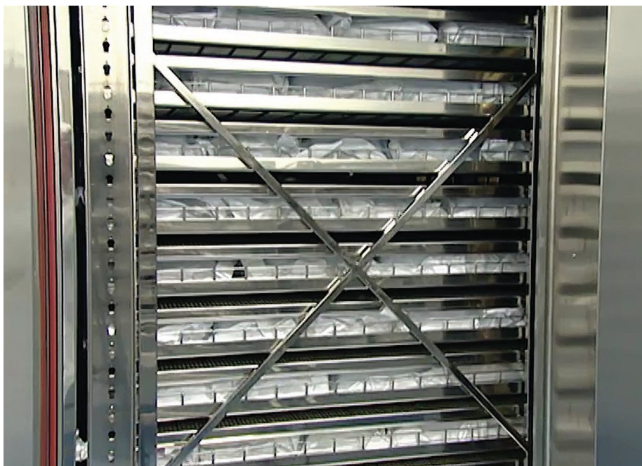
Figure 3: The autoclave used in steam sterilisation is equipped with an external jacket aimed to stabilise the conditions of temperature and pressure inside it across the entire sterilisation cycle. Saturated water vapour is blown inside.
