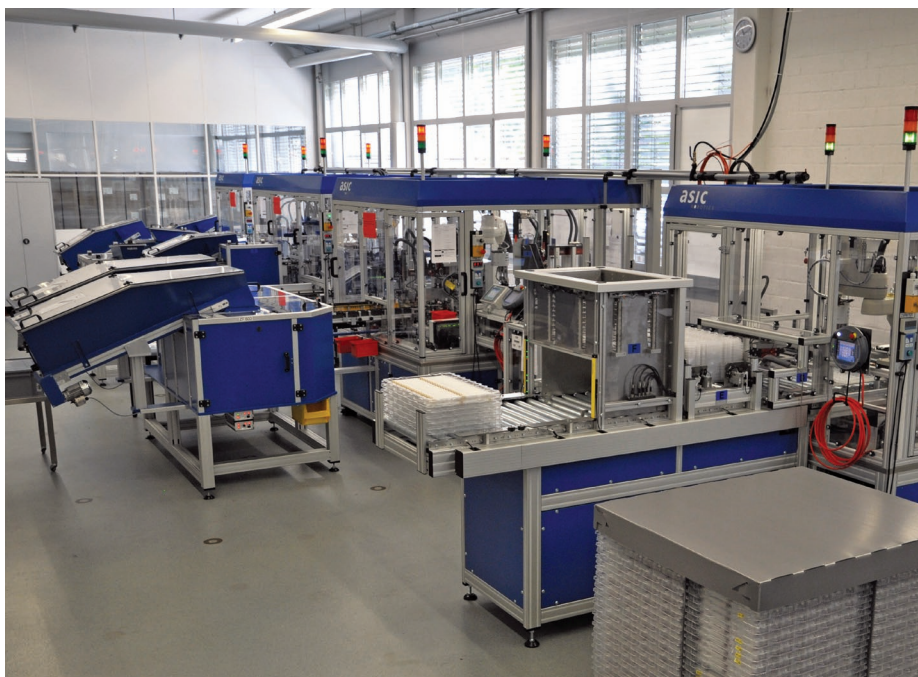
Figure 4: Flexible assembly line for fully customised YpsMate® auto injectors at one of Ypsomed's Swiss manufacturing sites.
