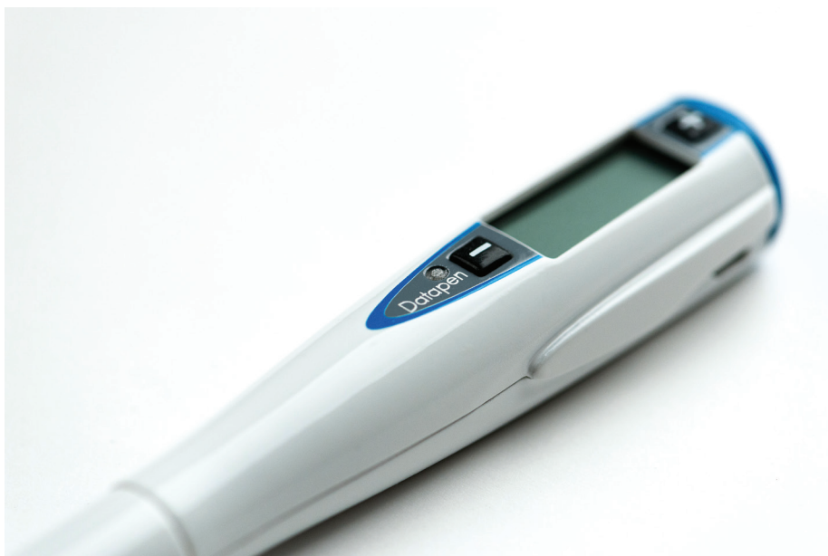
Figure 1: Biocorp's DataPen, a reusable injection pen connected to a smartphone app.
