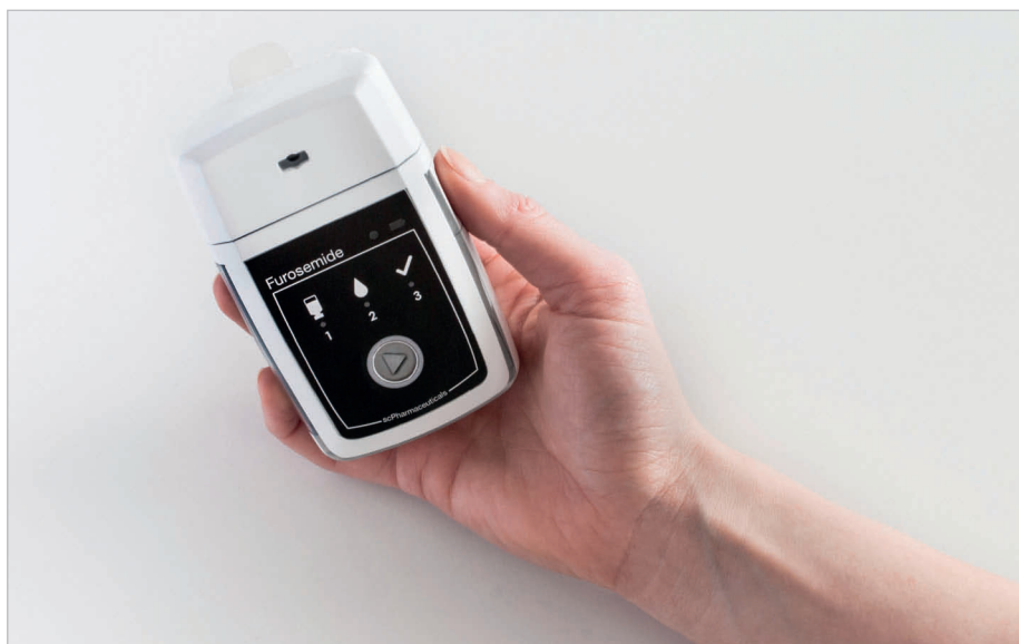
Figure 5: Now ready for use, the device is placed on the skin and the drug administered. After injection, disposable and reusable parts are separated and only the disposable is discarded.
