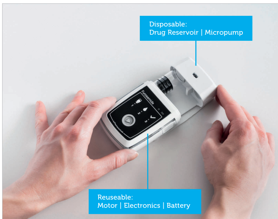
Figure 3: The Sensile pump is a customised delivery device. In this configuration, it consists of two major parts. In the disposable part, a micropump draws the product out of the reservoir and delivers it through a needle on the underside of the device (not shown). Key high-value components are retained for repeated use in the reusable part. During administration, only the disposable part is in contact with the drug or the patient. After injection, only the disposable is discarded.
