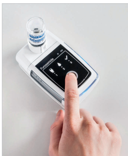
Figure 4: The patient transfers the drug from the vial into the device's internal reservoir. Upon completion of transfer, the vial is removed.
