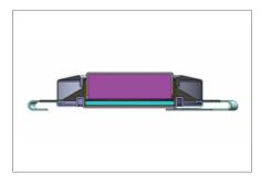
Figure 5: Schematic cross-section of the E-Cell.
