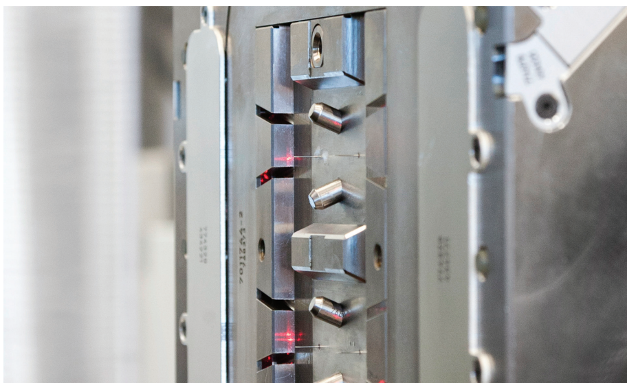
Figure 3: Cannula mounted in b-side of injection mould.
