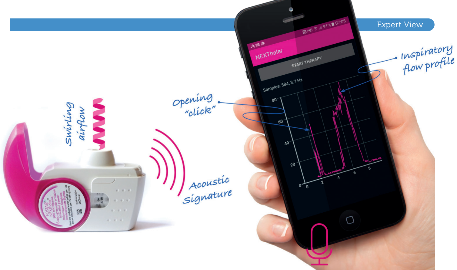
Figure 2: NEXThaler®: example of device connected to smartphone via non-electronic, audio communication. The app was developed by PA Consulting Group.
