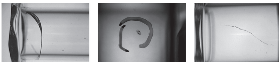
Figure 1: Characteristic glass defects in syringes: cracks, checks and scratches.
