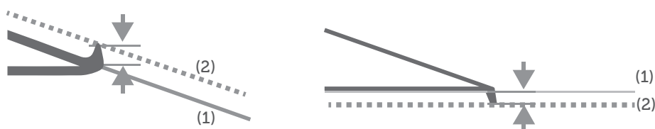
Figure 5: Dimensional inspection of the syringe needle.
