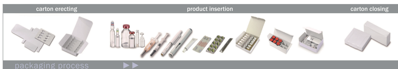
Figure 2: Main steps in the pharmaceutical packaging process.
