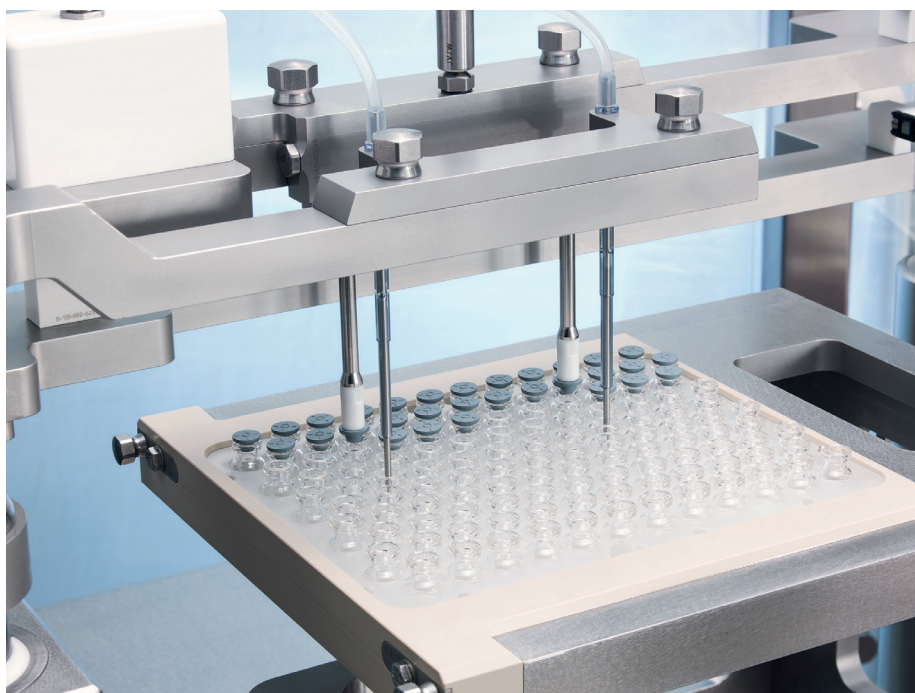
Figure 1: Filling of nested vials. (© Bosch)
