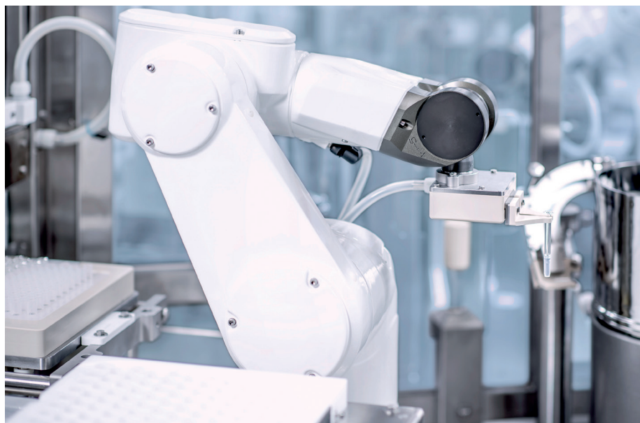
Figure 4: Fully automated robotic filling of syringes. (© Bosch/AbbVie)
