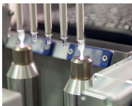
Figure 6: Luer cone bore plasma cleaning for baked on staked in needle syringe.
