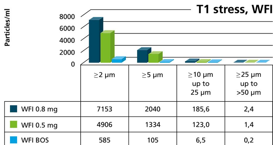
Figure 4: Sub visible silicone oil particles  $\geq 2 \mu\text{m}$  WFI solution.
