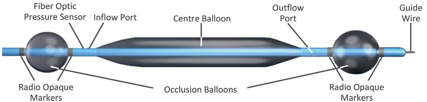
Figure 1: Schematic of the Occlusion Perfusion Catheter™.
