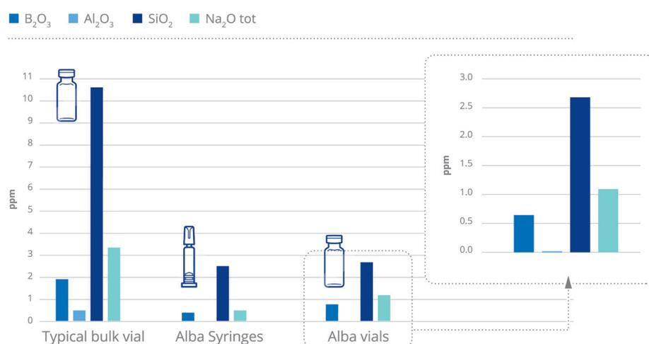
Figure 2: Alba vials inorganic extractables release performance in comparison with bulk vials and Alba syringes.
