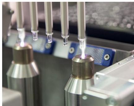
Figure 6: Luer cone bore plasma cleaning for baked on staked in needle syringe.
