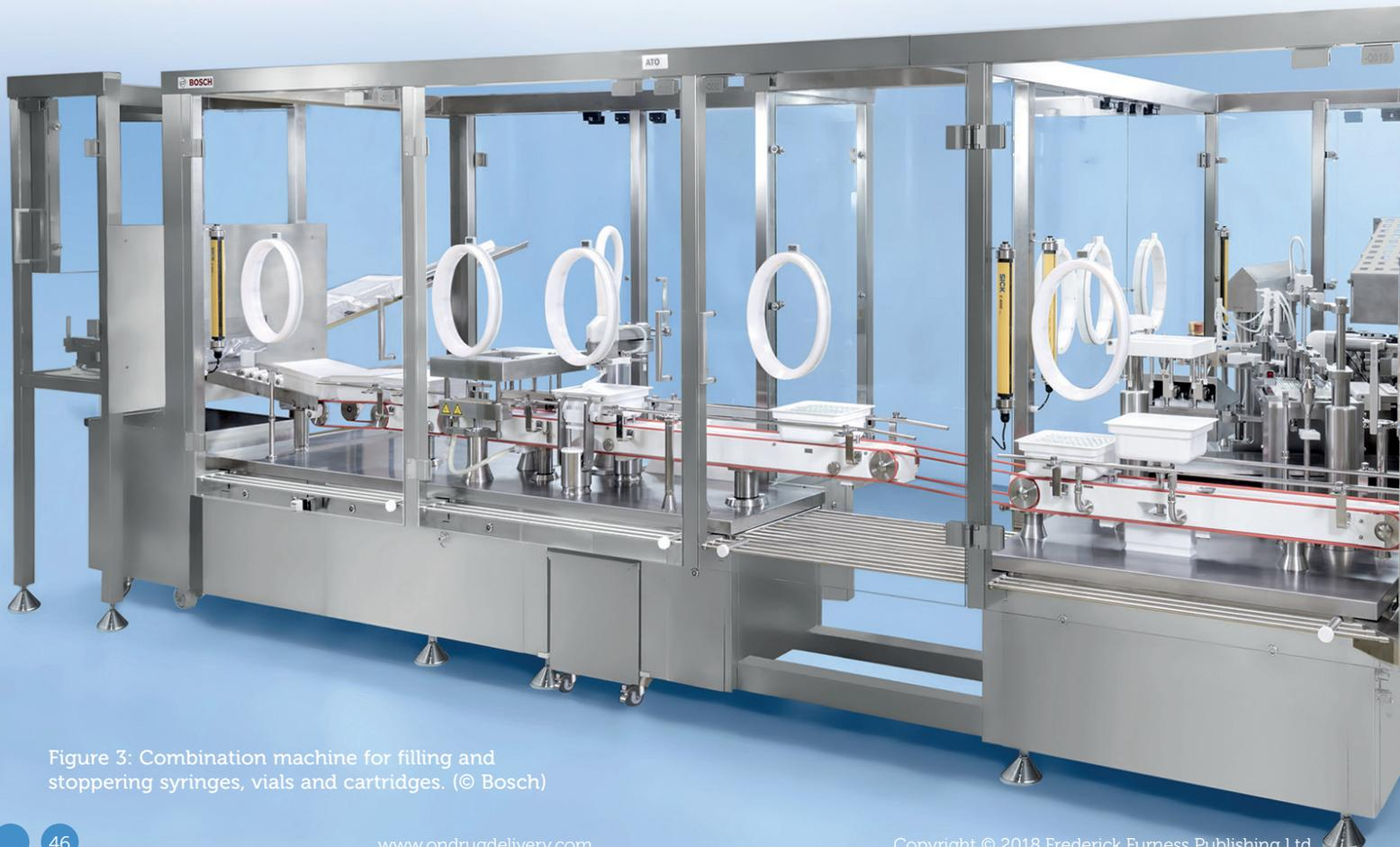
Figure 3: Combination machine for filling and stoppering syringes, vials and cartridges. (© Bosch)
