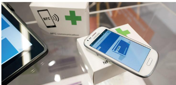
Figure 2: Rondo uses NFC chips integrated in the pack to improve patient communication. The NFC chip transmits its information as soon as a ‘read’ terminal is within range.
