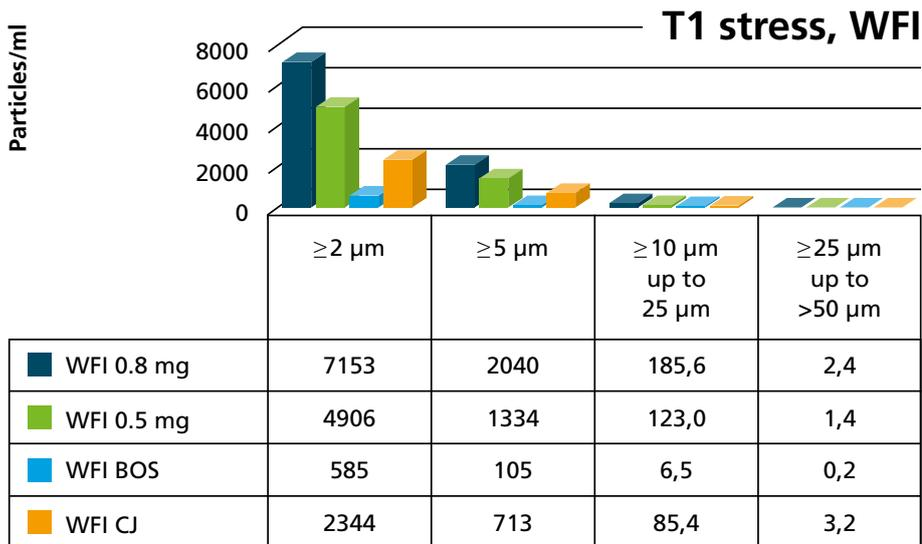
Figure 5: Sub-visible silicone oil particles  $\geq 2 \mu\text{m}$  Tween 80 0, 03% solution.
