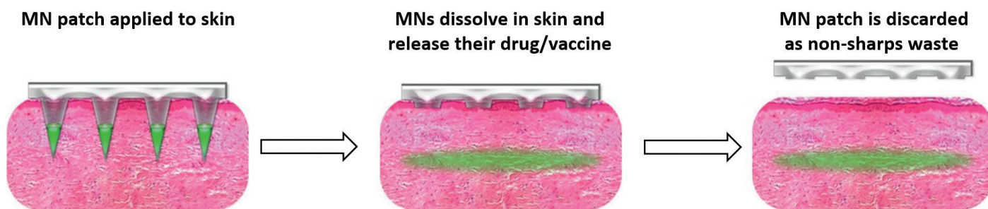
Figure 2: Schematic of Micron's patch showing microneedles dissolving and releasing their active in skin.
