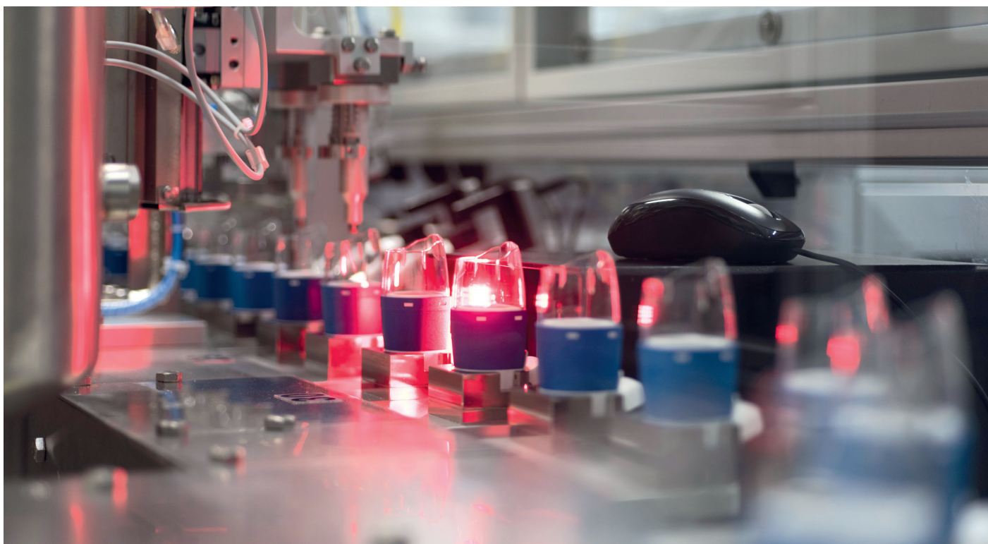
Figure 2: Integrated dose-counting actuator devices in testing.
