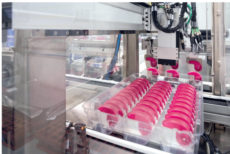
Figure 3: High-volume manufacture of dry powder inhalers.
