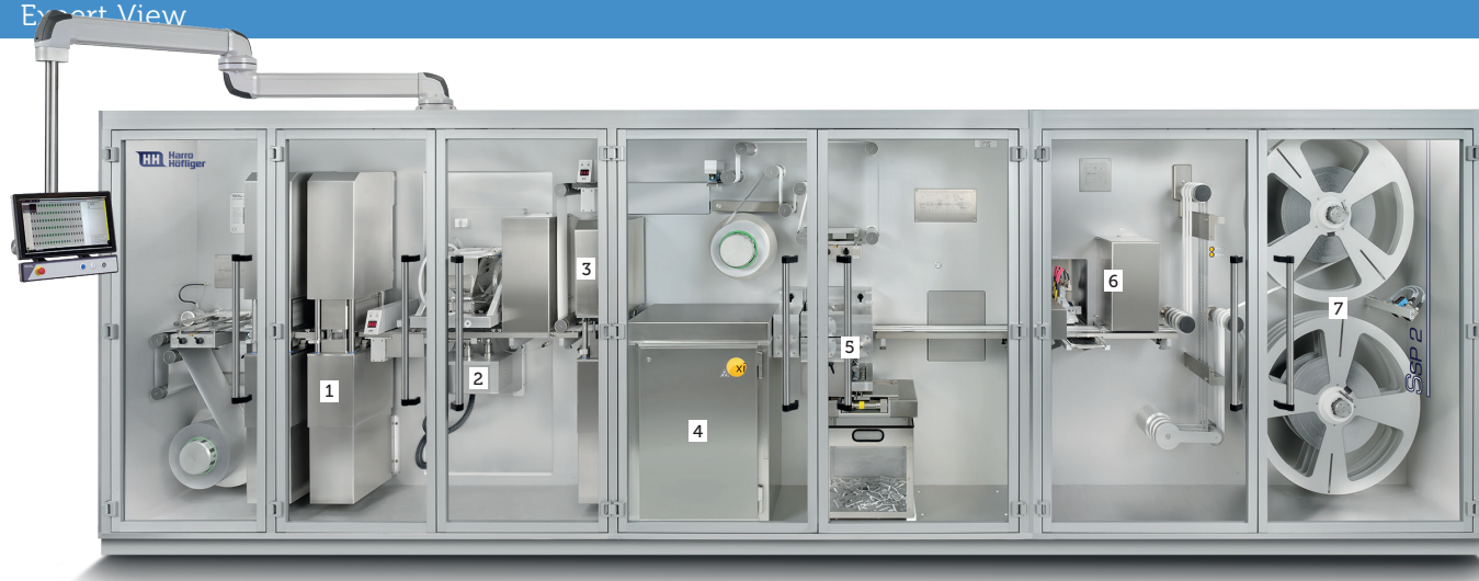
Figure 3: Machine for the manufacture of powder-filled blister strips: 1) Forming station; 2) Membrane filler; 3) Sealing station; 4) IPC X-ray module; 5) Longitudinal cutting; 6) Printing with camera control; 7) Winding.
