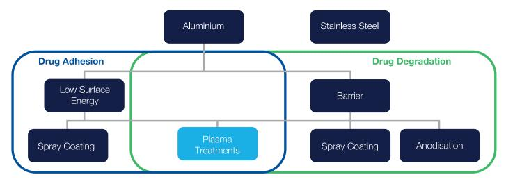
Figure 1: Types of surface treatment.
