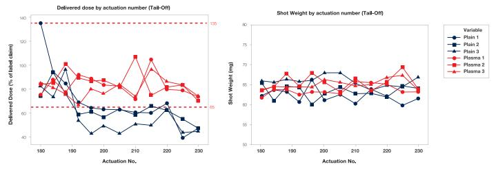
Figure 3: Tail-off characteristics for plasma-treated and plain canisters, using delivered dose testing (left) and shot weight (right), for a budesonide HFA suspension formulation.
