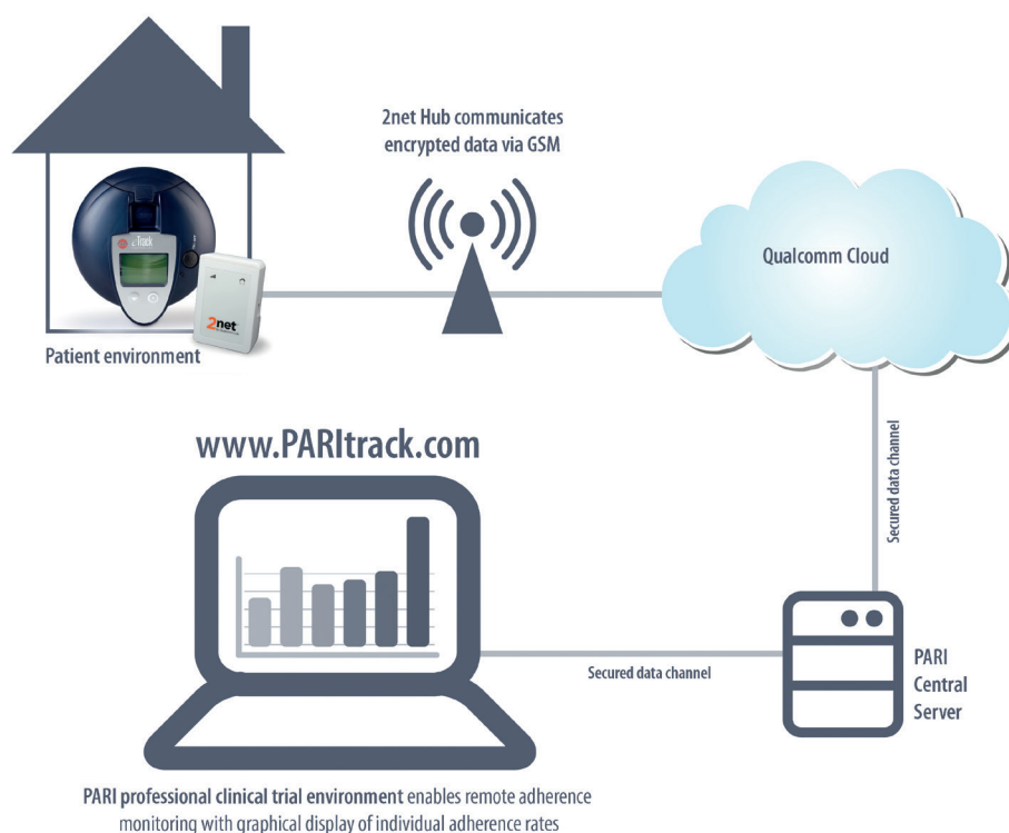
Figure 2: Set-up of data transfer from eTrack® Controller to PARIttrack® web portal.
