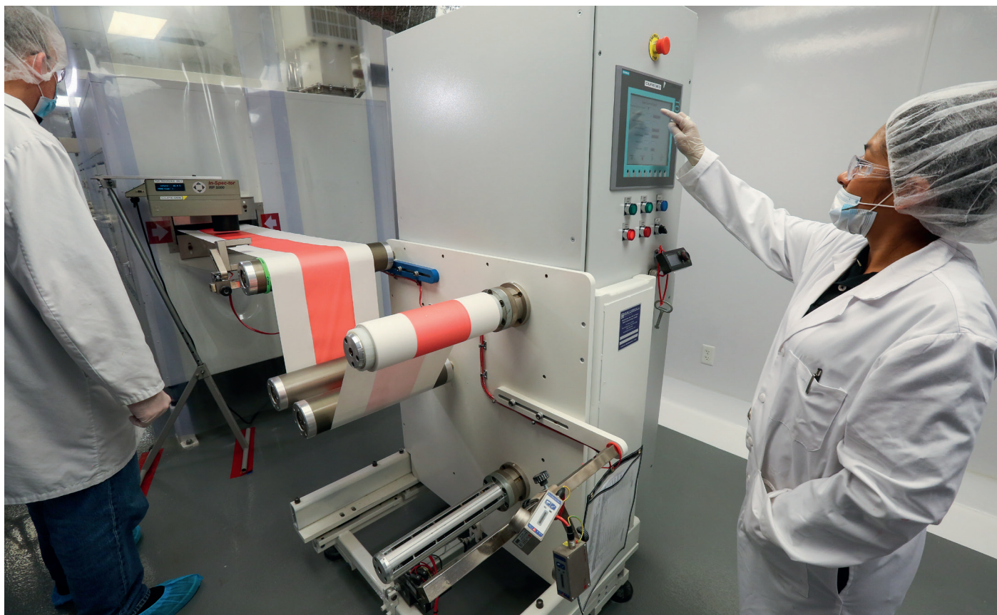
Figure 1: The film and liner exit the oven and are stored as master rolls, ready to be divided into daughter rolls and further into single doses.
