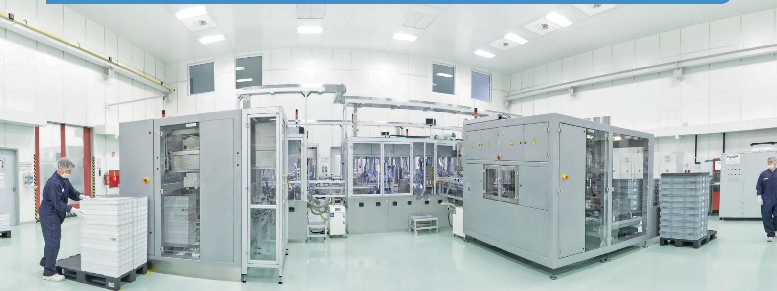
Figure 4: Fully automatic assembly line in an ISO 14644-1 Class 8 cleanroom.
