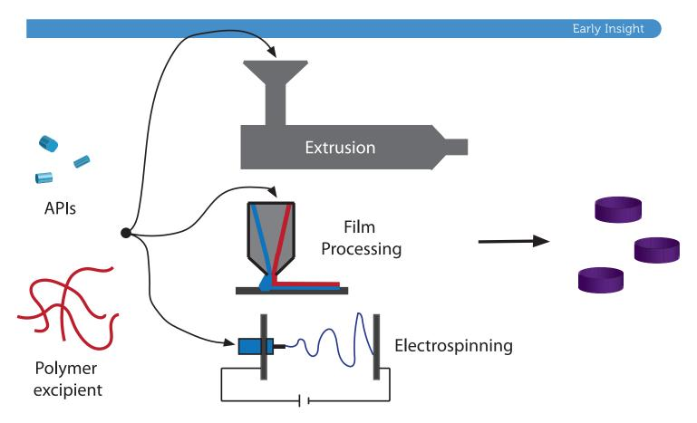
Figure 1: Downstream manufacturing processes for drug products inspired by polymer processing.
