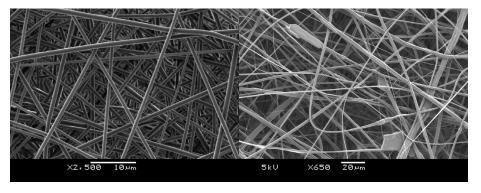
Figure 2: Electrospun fibres containing APIs: A) Amorphous API and B) Crystalline API.
