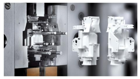
Figure 2: A hot runner mould.
