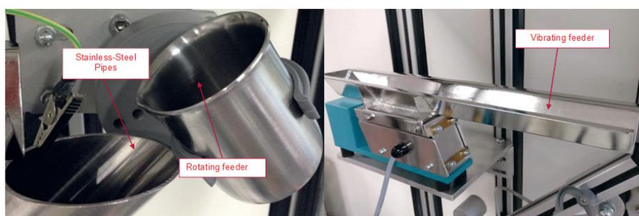
Figure 7: Vibrating/rotating feeder and stainless steel pipes.
