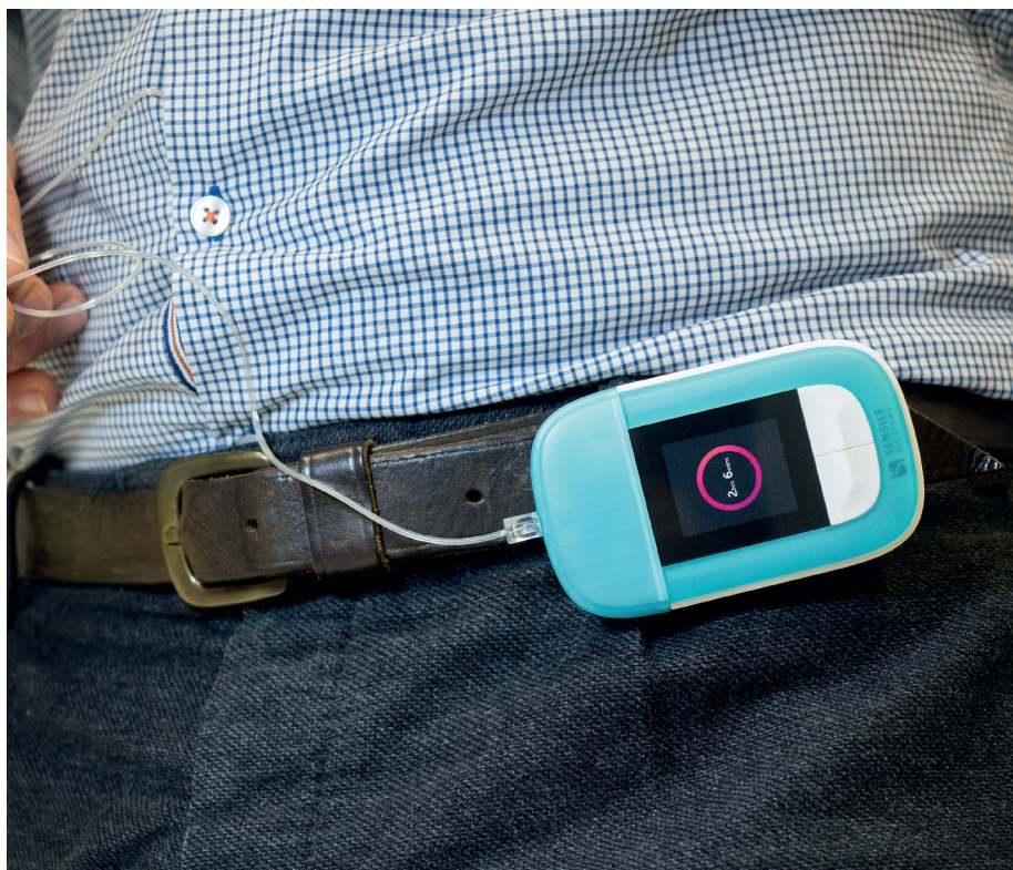
Figure 2: Sensile's belt-worn infusion pump.
