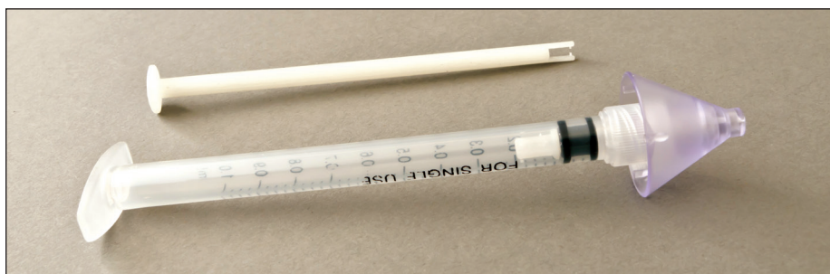
Figure 6: An Auto-disabled VaxINator™ device. Following complete drug administration the “catch” engages within the “latch”. If the plunger is retracted it will break off, leaving the device nonfunctional. Similarly if the atomizer is twisted off, the “catch” will either pull out the center of the atomizer or break off within the device.
