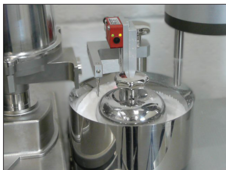
Figure 2: A typical powder bowl with ploughs and rakes to condition and aerate the powder.
