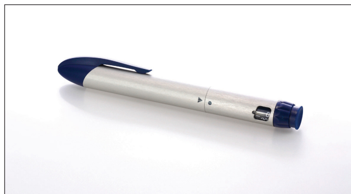
Figure 3: i-pen – re-usable, variable dose injection device designed with an intentionally 'non-medical' appearance.
