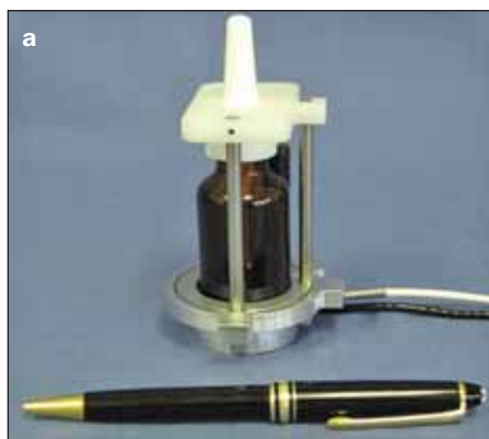
Figure 5: a) HAM with a load cell for electronic transfer of Hand Actuation Parameters to the actuator software. b) Travel and Force Curves obtained with the HAM Device
