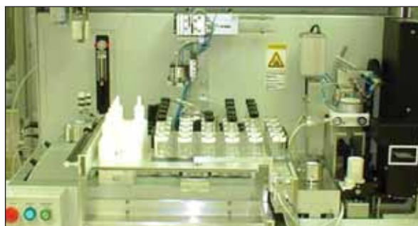
Figure 7: Fully automated system for Nasal Spray Dose Weight determination. In addition, subsamples are automatically prepared for Dose Content Uniformity testing
