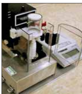
Figure 6: Pump Actuation Weight Station for automated dose weight determination of individual nasal spray pumps
