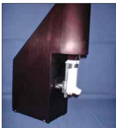
MDI-AS actuator. Product agitation via stepper motor at programmable angles
