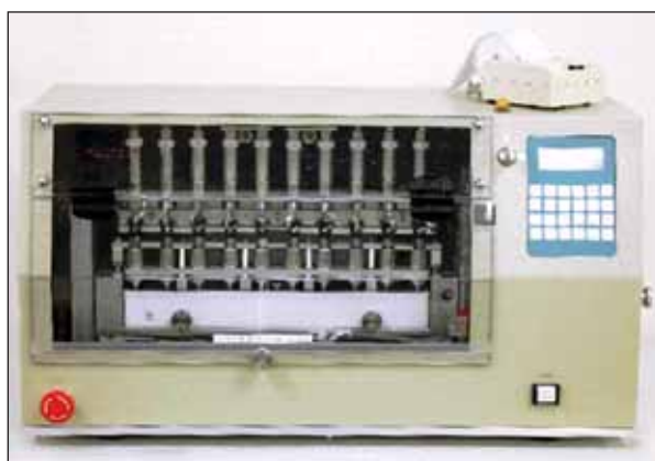
MDI FD-10 Repeated rotational or vertical shake followed by actuation of 10 MDI products
