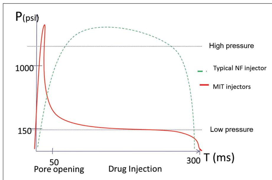
**Figure 2: Graph Comparing Injection Pressure Profiles of Needle-Free Injections (1 mL Water, 0.15 mm Nozzle).**
