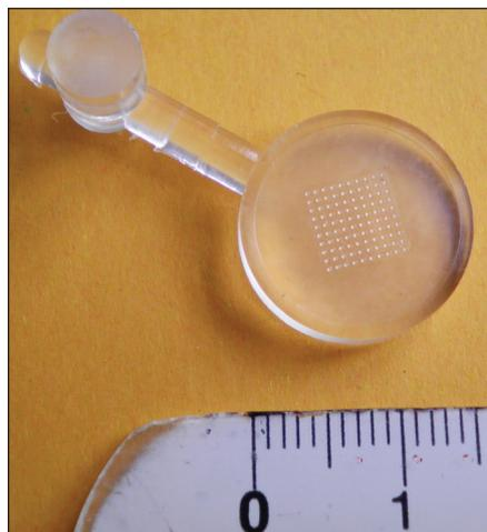
Figure 1: Prototypes of 100 micro-moulded microneedles made by Sirris Microfabrication Application Lab (Seraing, Belgium).
