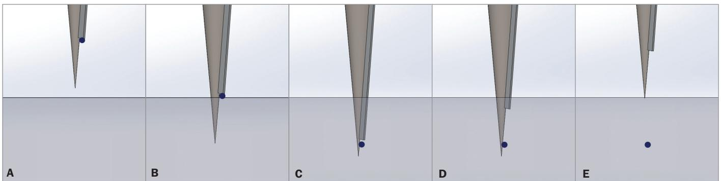
**Figure 2: Sequence of microneedle delivery via the Micropatch™.**
