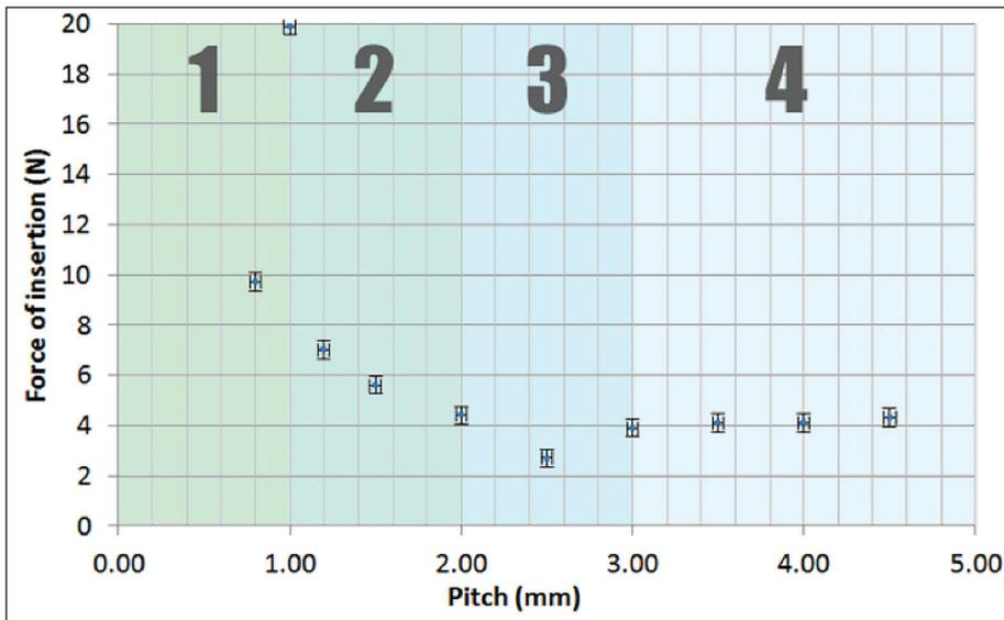
**Figure 5: Influence of needle density on insertion forces.**
