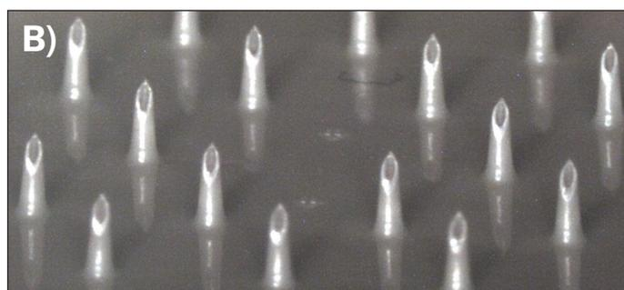
**Figure 1: A) Solid, drug-coated microneedles and B) hollow microneedle array. Solid microneedles are 250 $\mu$ m in length; hollow microneedles are 900 $\mu$ m tall. Both solid and hollow microneedles are moulded from medical-grade plastic.**
