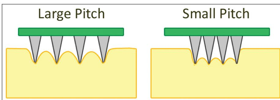
**Figure 6: The influence of spacing on needles' ability to pierce a membrane.**
