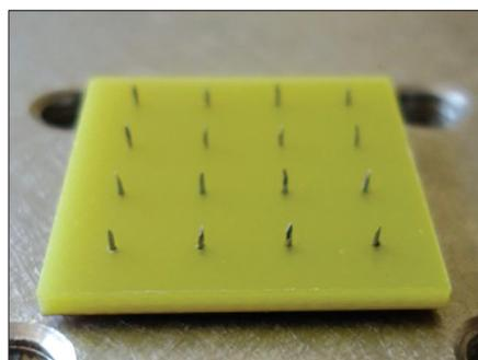
Figure 4: Picture of the microneedle array used in experiments.
