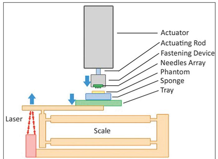
Figure 3: Principle of the test bench.
