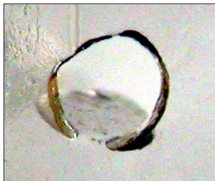
Figure 4: Capsules punctured in an Aventis Spinhaler®: A) Gelatin capsule; B) Quali-V-I, hypromellose, capsule. Capsules equilibrated at 35% relative humidity before testing.
