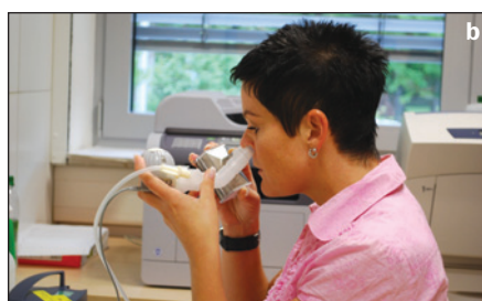
Figure 1: (a) PARI Vibrent®, a pulsating aerosol delivery prototype utilising a customised perforated vibrating membrane (eFlow platform nebuliser technology). (b) Use of the Vibrent during a deposition study using radiolabeled tracer. The nasal plug (resistance) was included in the output filter for capturing expelled aerosol.
