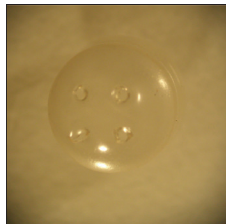
Figure 3: Capsule caps punctured in a Pharmachemie Cyclohaler® inhaler: A) Qualicaps gelatin capsule; B) Qualicaps Quali-V-I capsule. Capsules equilibrated at 35% relative humidity before testing.
