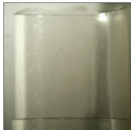
Figure 2: Capsule bodies cut open in an Aventis Eclipse® inhaler: A) Qualicaps gelatin capsule; B) Qualicaps Quali-V-I capsule. Capsules equilibrated at 35% relative humidity before testing.
