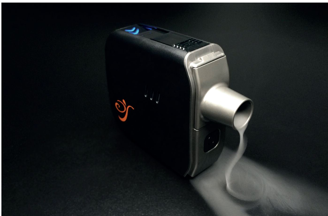
Figure 1: The Dance-501 insulin inhaler uses a vibrating mesh to create a soft mist.
