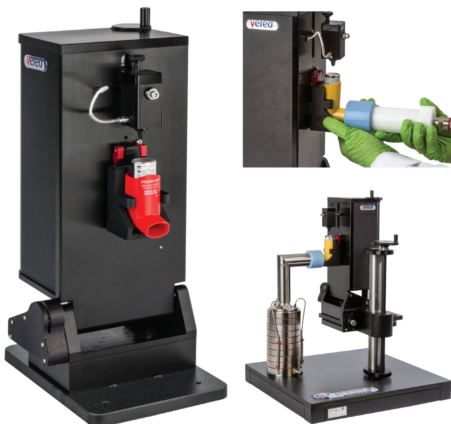
Figure 3: Proveris Vereo SFMDx actuator for pMDI products (left); SFMDx with DCU setup (top right) and Anderson Cascade Impactor (bottom right).
