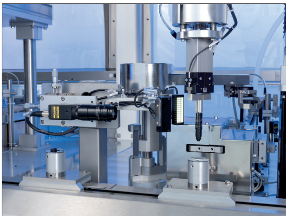
Figure 3: A camera system checks for completeness and correct settings of all parts.
