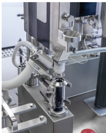
Figure 2: Fill2Weight™ Powder Dispensing Systems inside an aseptic isolator.
