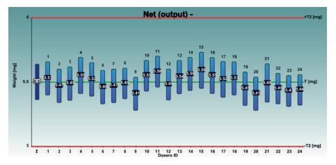
Figure 4: Inhalac 251 + 4% Lactose microfine, behaviour of the 24 dosators on Adapta.
