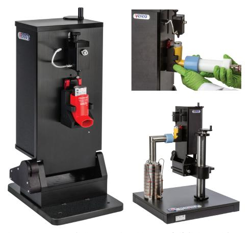
Figure 3: Proveris Vereo SFMDx actuator for pMDI products (left); SFMDx with DCU setup (top right) and Anderson Cascade Impactor (bottom right).
