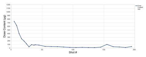
Figure 2: Variable dose delivery from a pMDI device due to lack of shaking.
