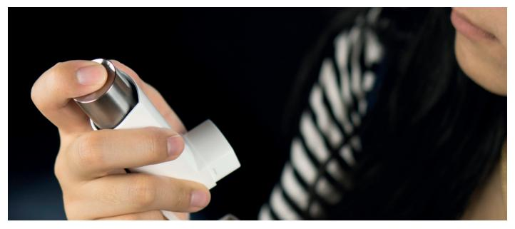
Figure 1: MDI training device designed to replicate an actual MDI's form factor and operation while providing the user with multisensory feedback.
