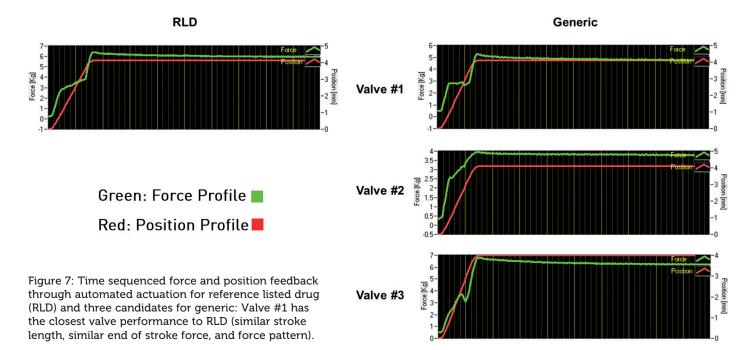
represents the device's resistive force during the actuation. Moreover, this signature force profile for each device type can be used to determine the product actuation force in Viota. The differences in product actuation force across multiple products also help characterise the ease of use for specific patient populations (e.g. children and older patients).
