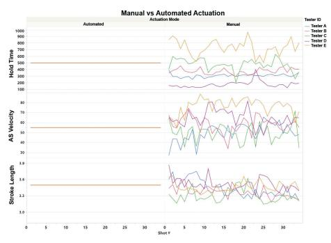
Figure 1: Consistent control over actuation parameters with automated actuation (left) and variation observed with human actuation for pMDI devices (right).
