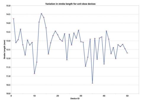
Figure 8: Stroke length differences in unit dose devices from the same lot.
