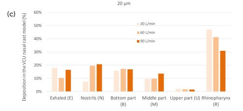
Figure 3: Deposition in the nasal cavity model expressed in term of total drug delivered in the nasal cavity (N+U+M+B+E+R) for 3  $\mu$ m (A), 12  $\mu$ m (B) and 20  $\mu$ m (C) (n=3).
