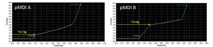
Figure 6: Force displacement graphs from two different pMDI products obtained from Viota software.
