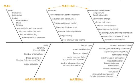
Figure 3: The complexity and manual nature of cascade impaction means that that are many potential sources of variability.<sup>5</sup>
