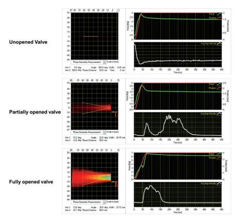
Figure 4: Comparison across plume geometry measurements between an unopened valve, partially opened and a fully opened valve.
