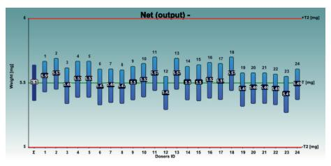
Figure 5: Respitose SV003 + 4% Lactose microfine, behaviour of the 24 dosators on Adapta.
