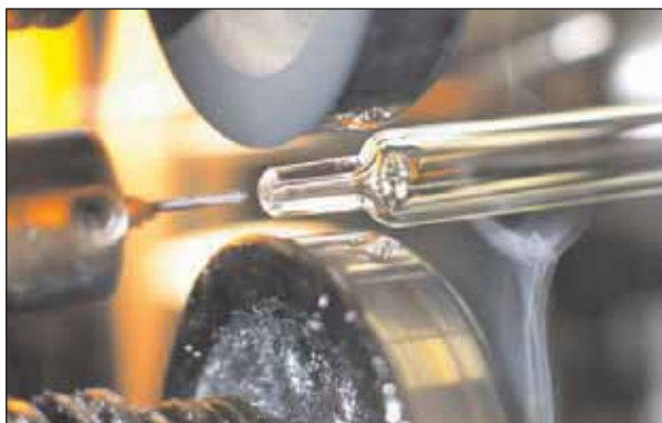
Figure 9: Pin used for forming the cone bore
