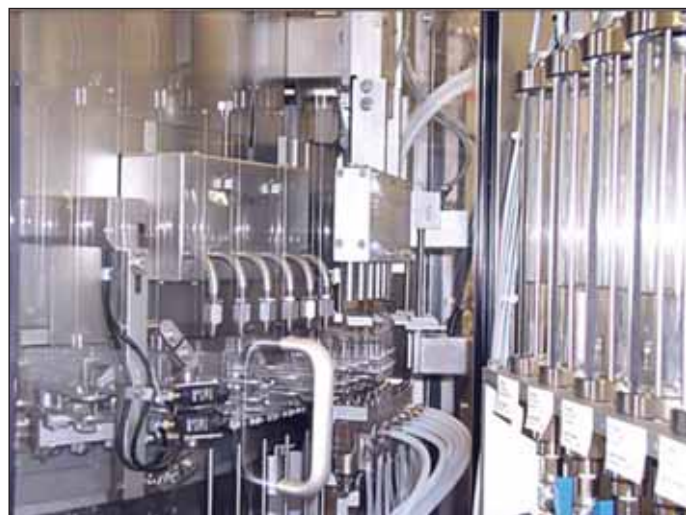
Figure 2: Syringes are washed with water for injection
