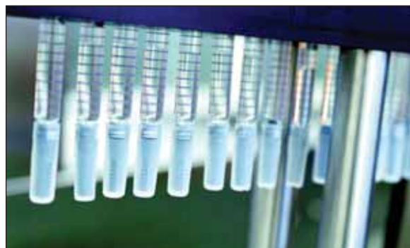
Figure 5: Aseptically prefilled syringes leave the filling machine
