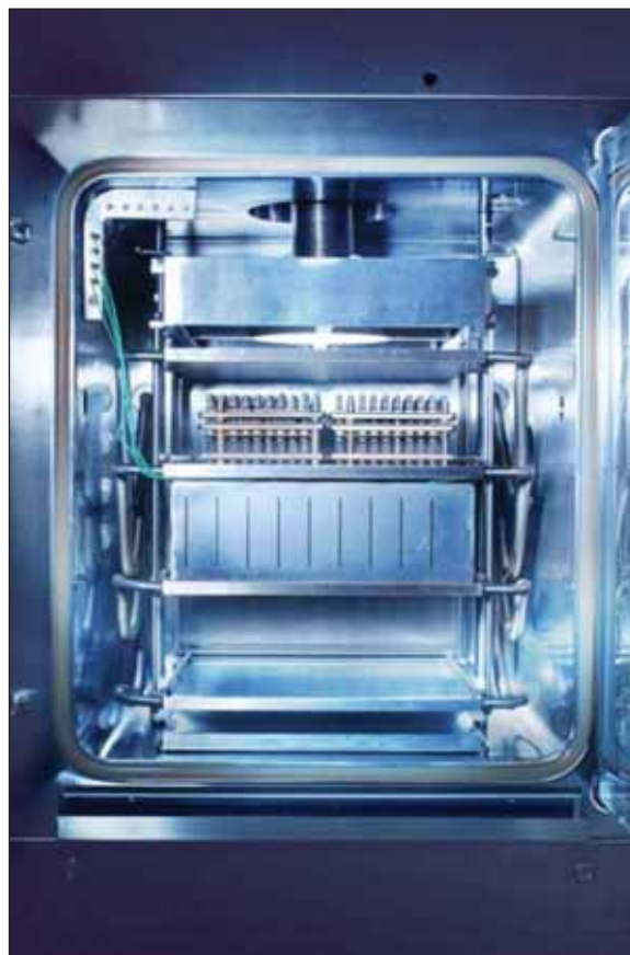
Figure 2: Inner view of Vetter's state-of-the-art laboratory freeze-dryer
