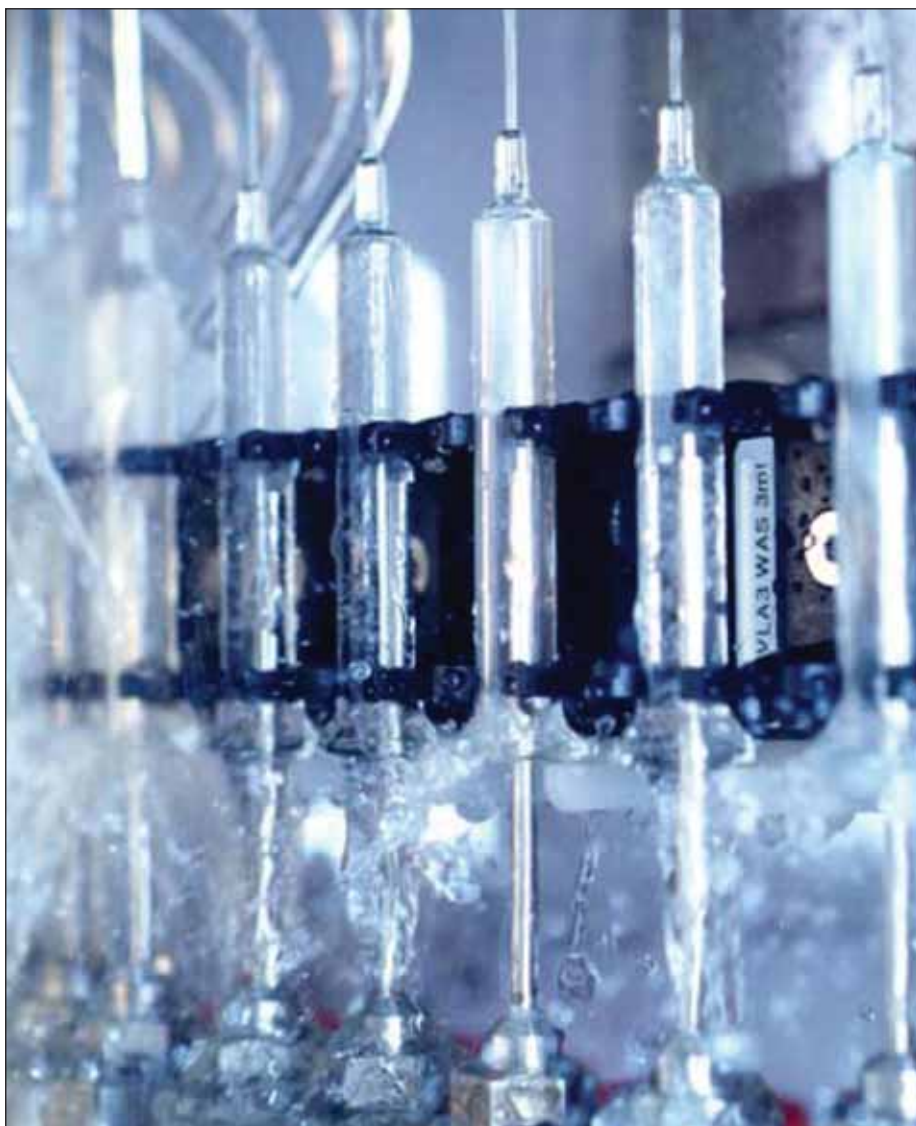
Figure 3: Validated cleaning processes. The washing process enables high quality in the manufacturing of aseptically prefilled application systems
