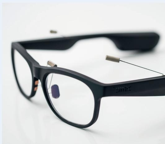
concept which integrates wireless eye-tracking technology into a standard pair of eyeglasses. The smart glasses use electro-oculograms, which measure the electric potential across particular points on the skin around the eyes during eye movement. The glasses use five dry-contact electrodes developed by Datwyler.
