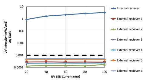
Figure 6: The results of the experiment showing UV reach.
