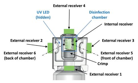
Figure 5: The experimental set-up to determine UV reach.
