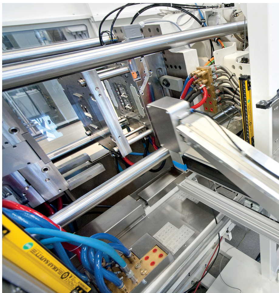
Figure 3: If the Z.NFS is integrated into the Z.BLIZZARD as shown here, it is an integrated system that guarantees the highest level of purity in the production process, as there is no human touch and the process can be carried under cleanroom conditions.
