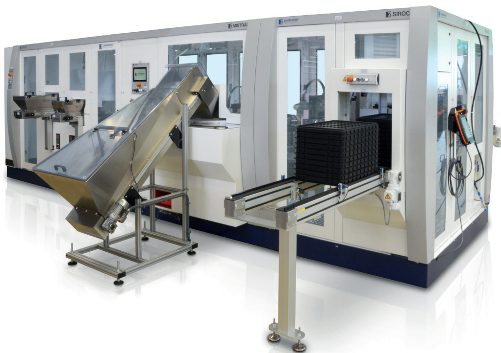
Figure 4: If the Z.BLIZZARD is still connected to the Z.MISTRAL, which is responsible for the downstream, and the palletising system Z.LODOS, it is possible to cover the complete process chain, from the granulate to the finished packed PFS.
