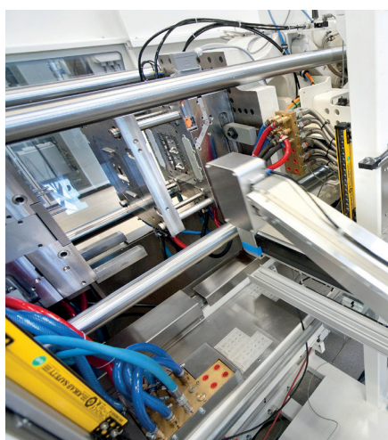
Figure 3: A detailed view: The Z.NFS needle separating system can separate 4– 32 needles or cannulas with up to 12 cycles per minute. Currently, diameters from 0.2 mm and lengths up to 45 mm can be processed.
