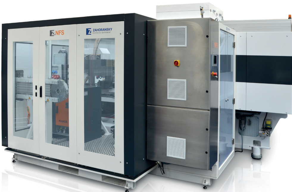
Figure 1: The Z.BLIZZARD produces ready-to-fill PFS from COC/COP polymer with a very long autonomy time.
